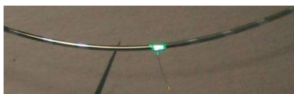
Fig. 2. Optical micrograph of a flexed fiber with a 1 mm long green emitting OLED (Copyright WILEY-VCH Verlag GmbH & Co. KGaA, Weinheim).
