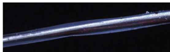
Fig. 3. (Top) Schematic picture of the double wire organic solar cell (Bottom) Optical micrograph of a polymer-clad double wire solar cell (Copyright by the American Association for the Advancement of Science).
